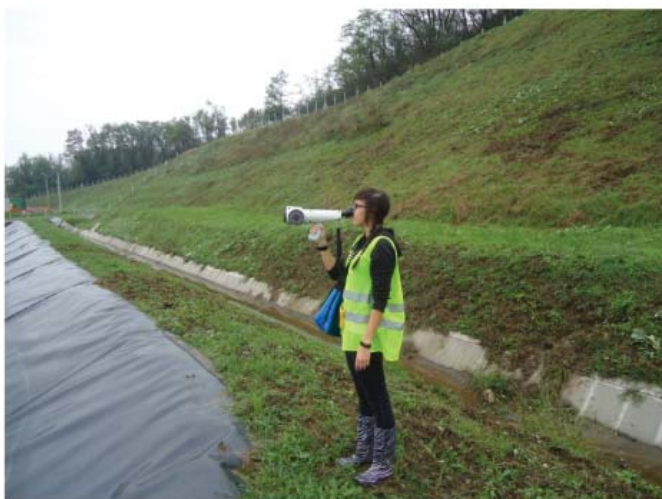
Picture 3: The use of Nasal Ranger field olfactometer for odour measurement (photo: Kálmán Samu-Nagy, Nóra Koplányi)
