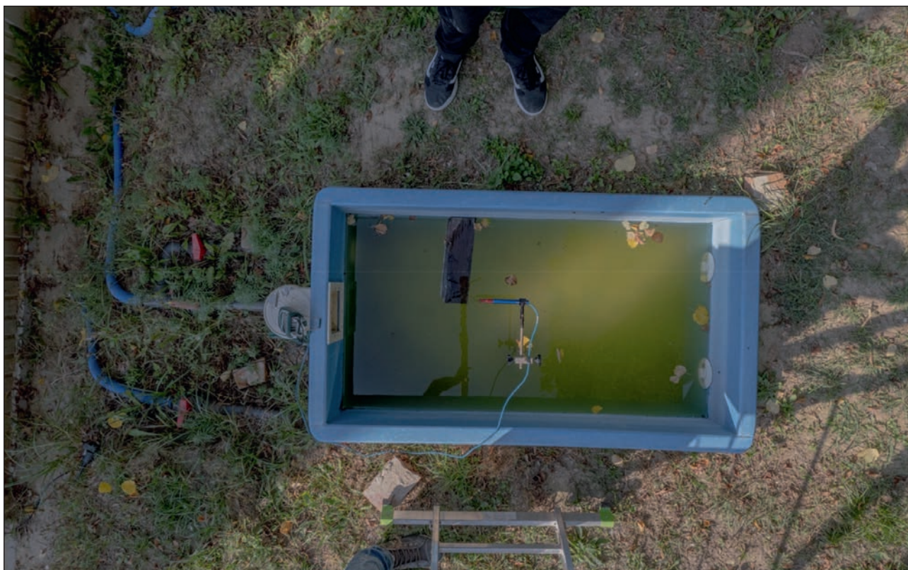
Figure 3: Nadir image by the DJI AIR S2 UAV from the altitude of 2 metres, a wind speed sensor placed in the pool.
